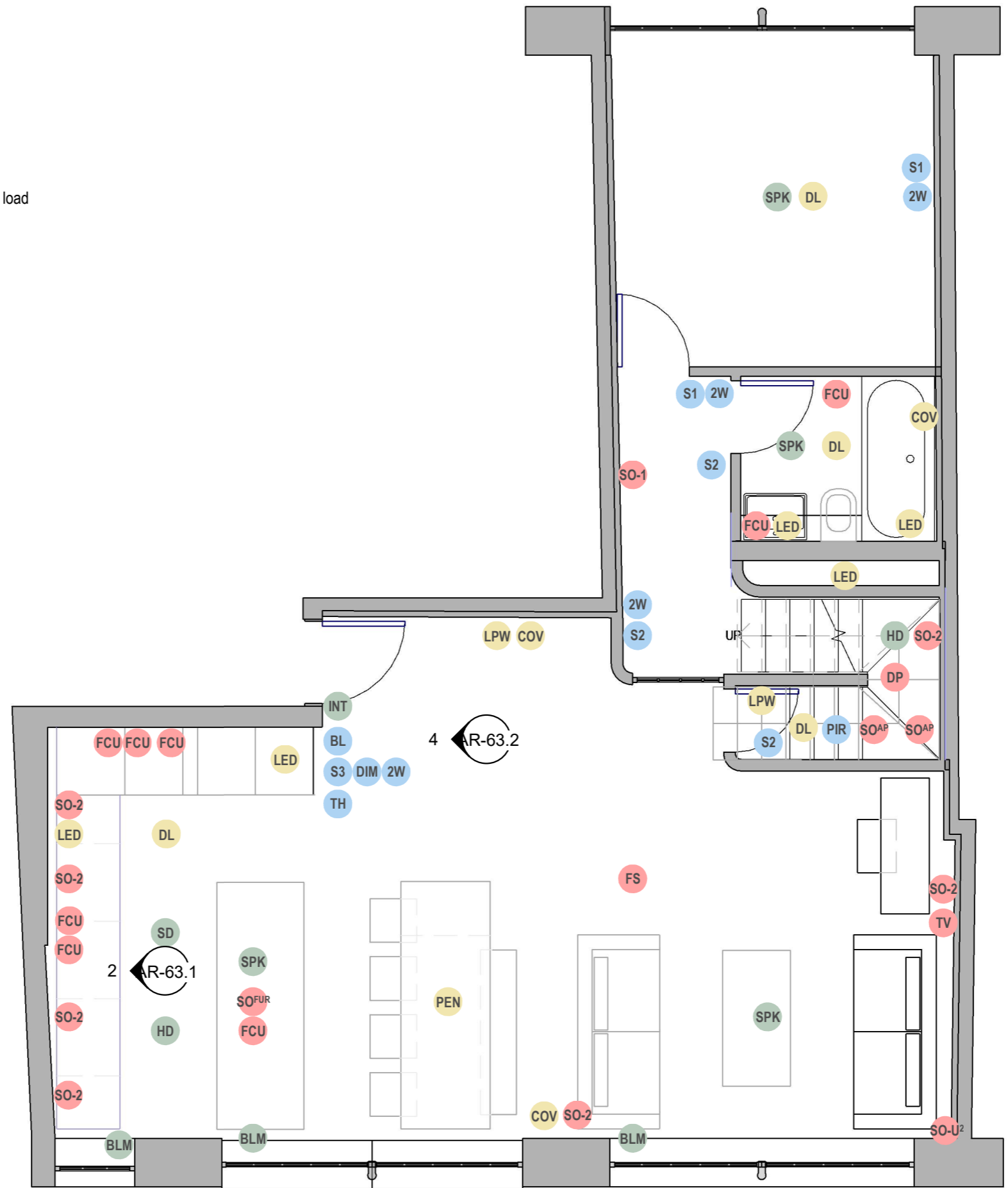
1 Electric Plan Ground Floor 1 : 50
